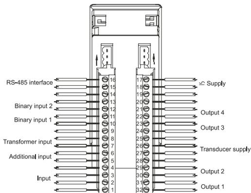
Fig. 1. View of controller connection terminal strips.
