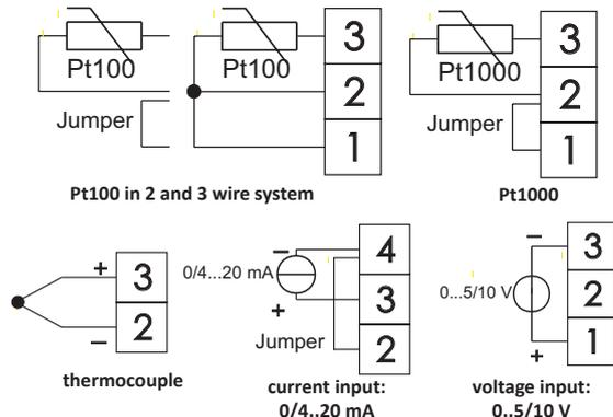
Fig. 2. Connection of input signals.
